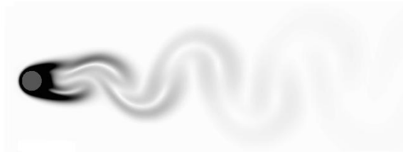
Figure 4: Temperature gradient visualization for the static cylinder at Re=100 .
