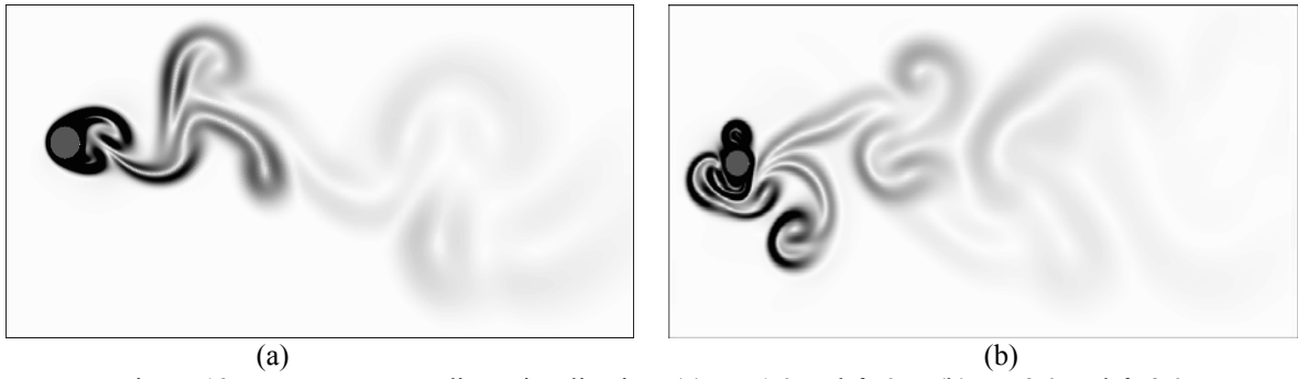
Figure 12: Temperature gradient visualization, (a) U_r=1.0 and f_r=0.5 ; (b) U_r=2.0 and f_r=2.0
